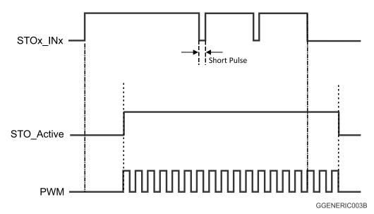
Figure 13: Timing Diagram of short pulses
