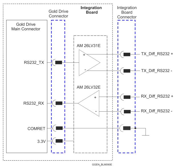
Figure 65: Differential RS232 Interfacing
