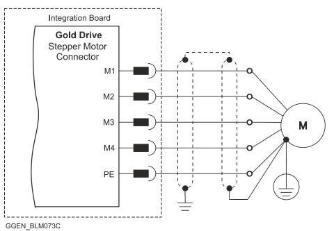
Figure 11: Stepper Motor Power Connection Diagram
