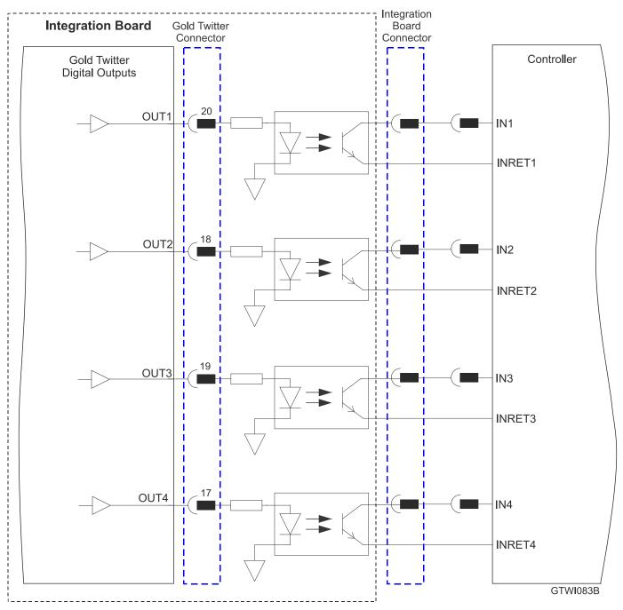
Figure 53: Digital Output 5V and 3.3V Level Mode Connection Diagram
