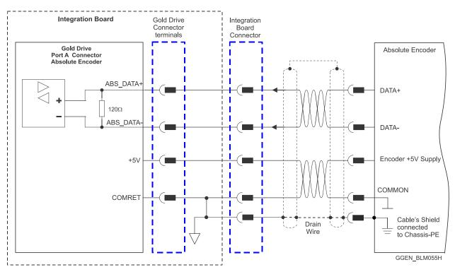
Figure 30: Absolute Serial Encoder – Recommended Connection Diagram for Pansonic, Tamgawai, Sanyo / Nikon
