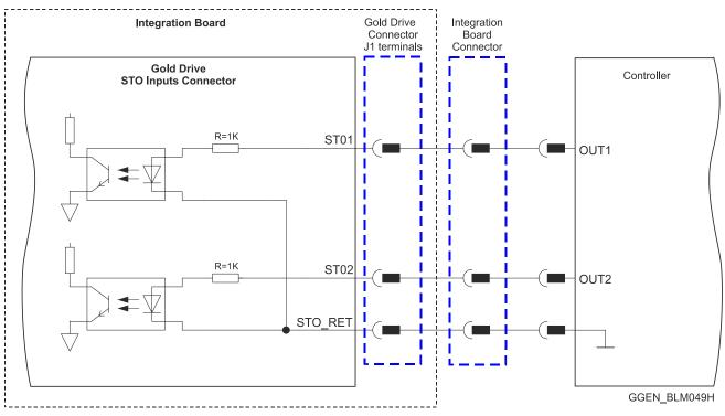
Figure 15: STO Input Connection – TTL Option
