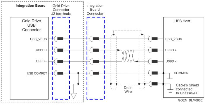
Figure 56: USB Network Diagram
