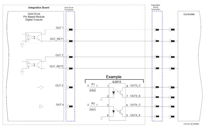
Figure 43: Digital Output Connection Diagram – TTL Connection
