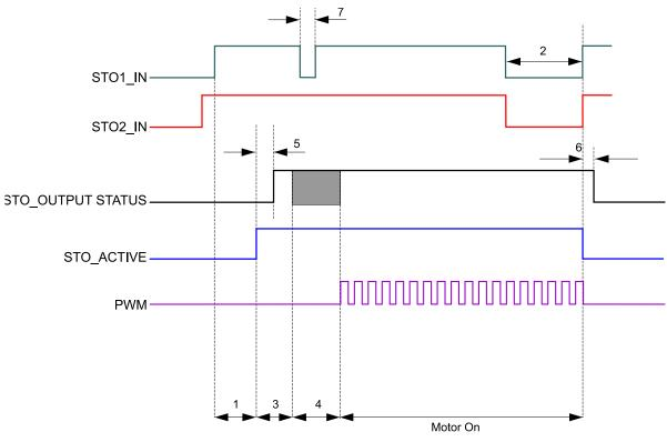
Figure 23: STO Timing Diagram
