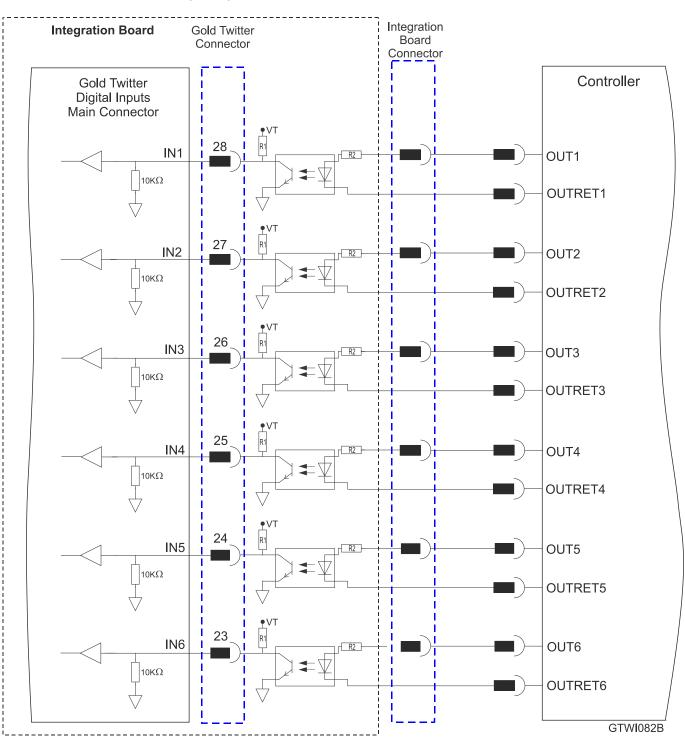
Figure 52: Digital Input 5V Logic level Mode Connection Diagram
