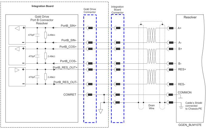
Figure 35: Port B – Resolver Connection Diagram
