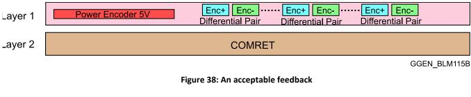
The following is an example of a Feedback with inner return layer, but is not recommended.
