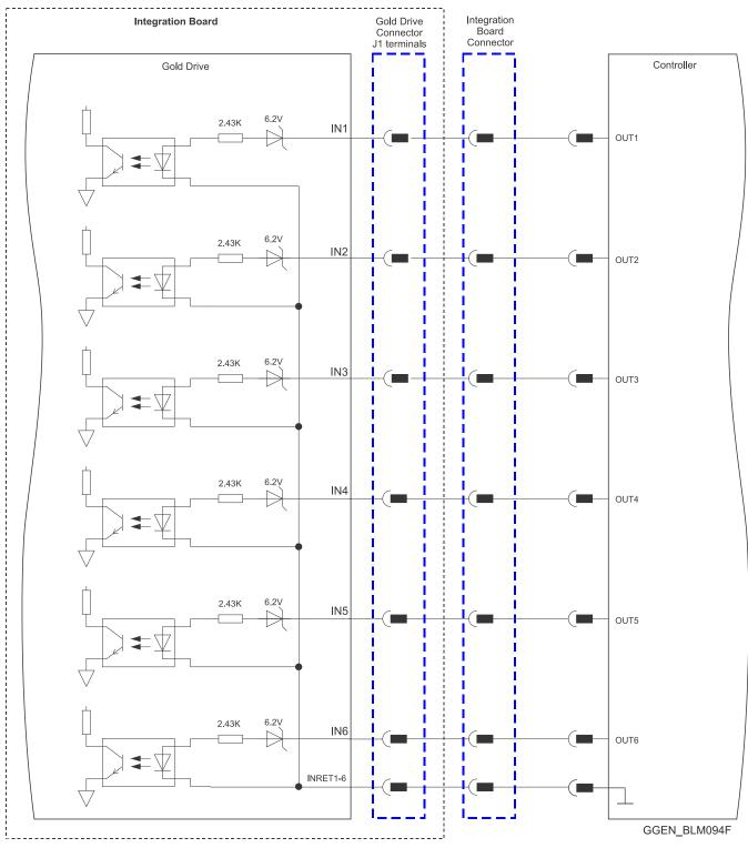
Figure 47: Digital Input Source Mode - PLC voltage level Connection Diagram
