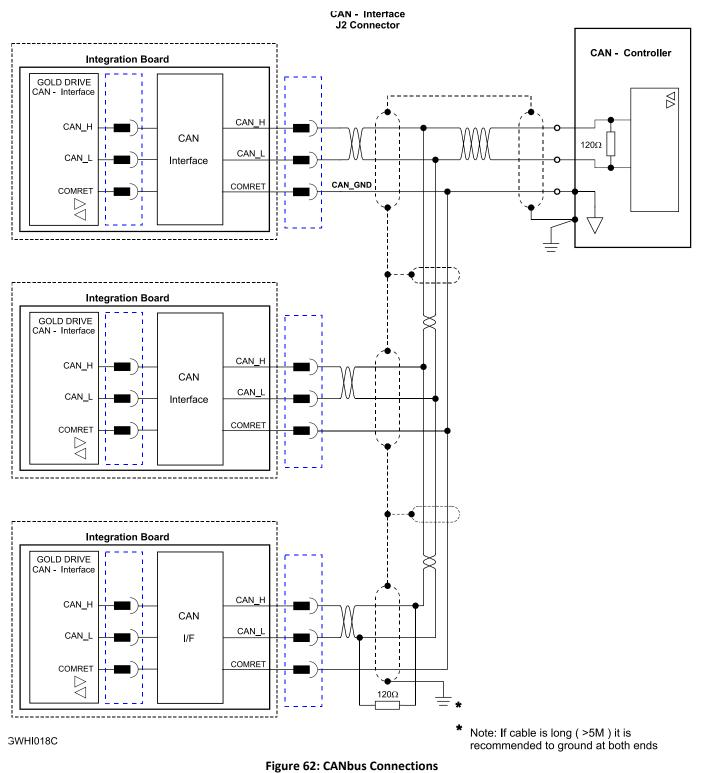
A 120  $\Omega$  termination resistor should be connected at each end of the network
