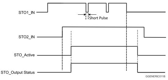
Figure 21: STO Output Status Timing Diagram
