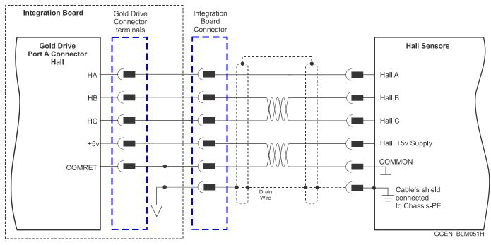
Figure 28: Hall Sensors Connection Diagram
