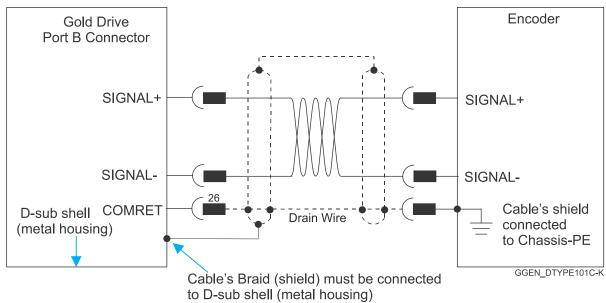
Figure 5: Feedback Port A and B Cable Assemblies
