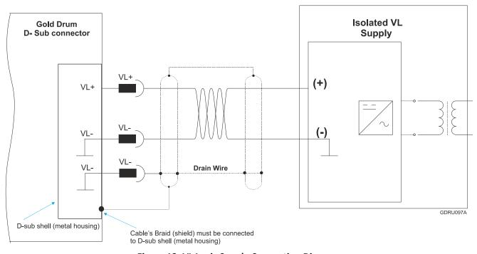
**Figure 13: VL Logic Supply Connection Diagram**
