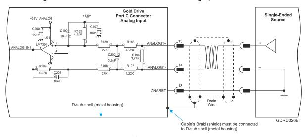
Figure 23: Differential Analog D-Type Input
