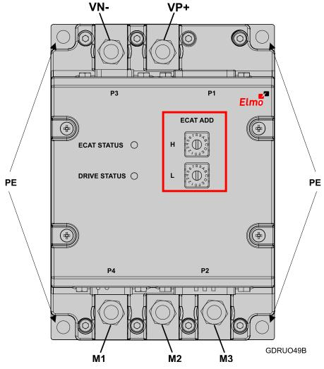
**Figure 37: EtherCAT Address Switches**
