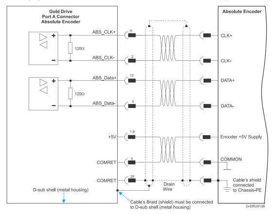
Figure 17: Absolute Serial Encoder – Recommended D-Type Connection Diagram for EnDAT,
