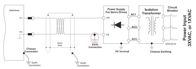
Figure 12: Isolated from the Mains DC Power Supply connection
