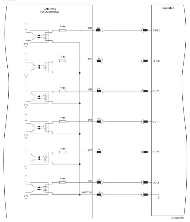
Figure 28: Digital Input TTL Mode D-Type Connection Diagram
