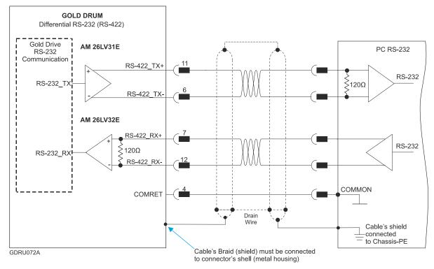
Figure 40: RS-422 (Differential RS-232) Communication Connection Diagram
