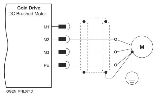
**Figure 10: DC Brushed Motor Power Connection Diagram**
