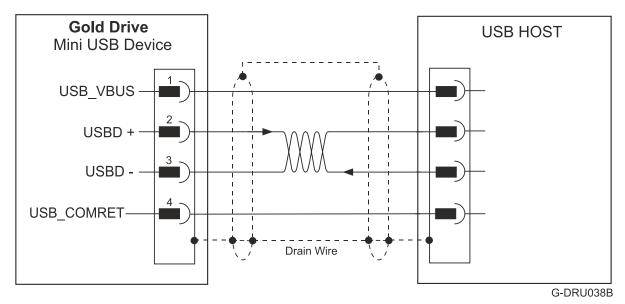
Figure 34: USB Network Diagram
