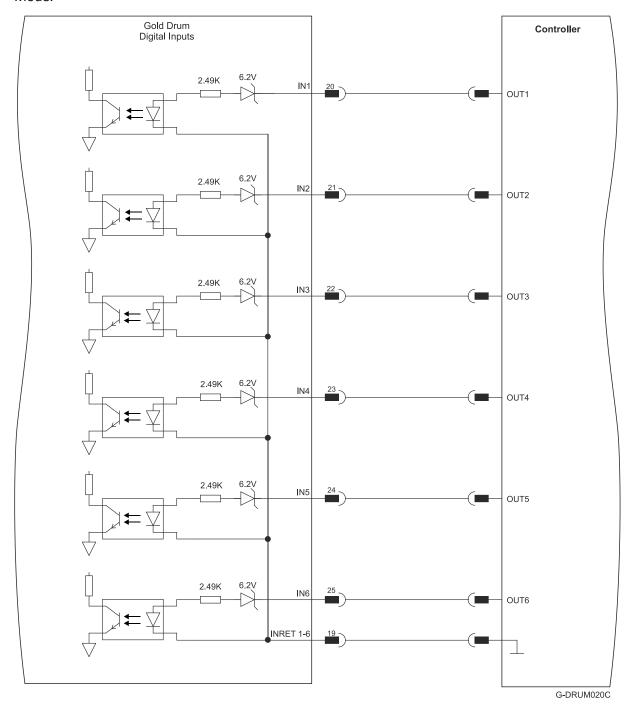
Figure 30: Digital Input D-Type Connection Diagram - Source PLC Option
