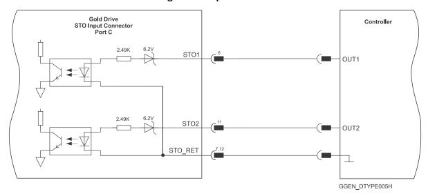
Figure 24: STO D-Type Input Connection – PLC Source Option
