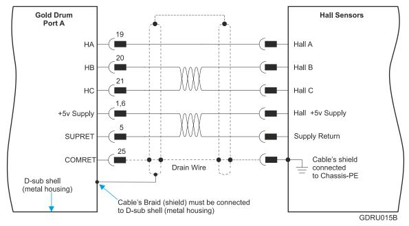
Figure 16: Hall Sensor Connection Diagram
