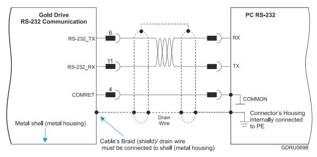
Figure 39: RS-232 Connection Diagram Example
