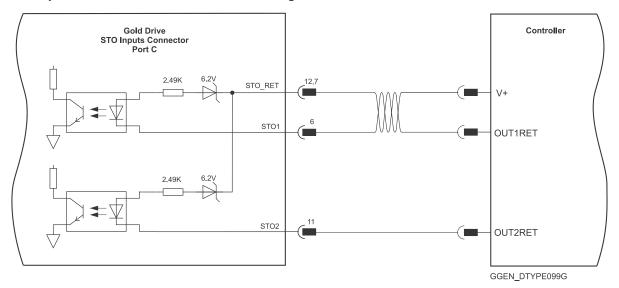
Figure 26: STO D-Type Input Connection – Sink Option
