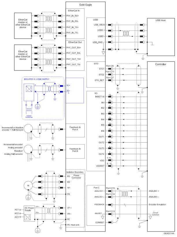
Figure 2: Gold Eagle Connection Diagram - EtherCAT
