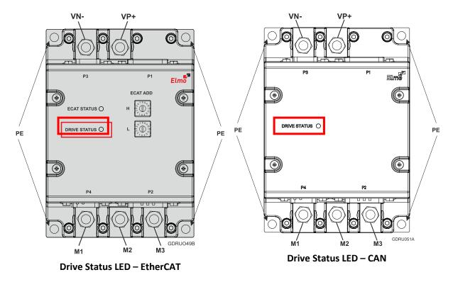
Figure 14: Drive Status LEDs
