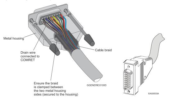
Figure 4: D-Type Cable Assemblies
