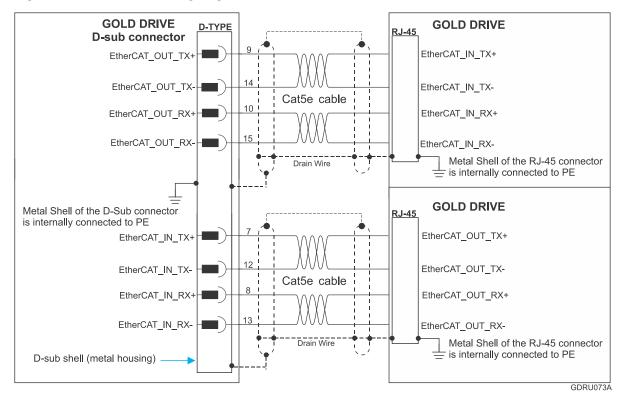
Figure 35: EtherCAT with D-Type Connections
