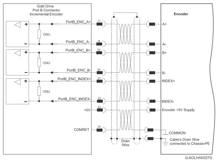
Figure 20: Port B Incremental Encoder Input – Recommended Connection Diagram
