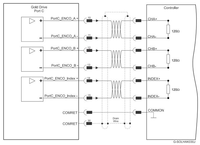
Figure 23: Encoder Differential Output – Recommended Connection Diagram
