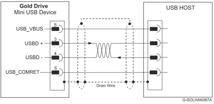
Figure 35: USB Network Diagram
