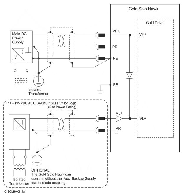
Figure 12: Separate Control Supply Connection Diagram
