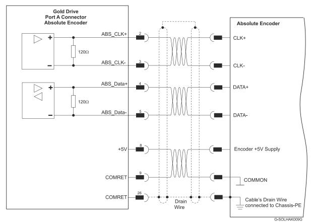
Figure 17: Absolute Serial Encoder – Recommended Connection Diagram for EnDAT, Biss, and SSI
