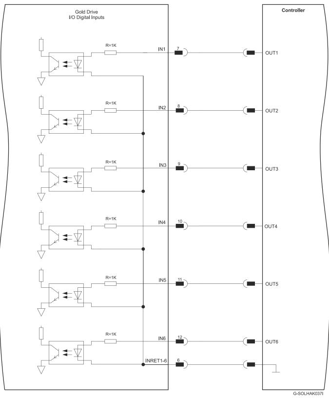
Figure 25: Digital Input TTL Mode Connection Diagram
