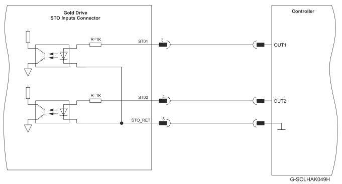
Figure 32: STO Input Connection – TTL Option
