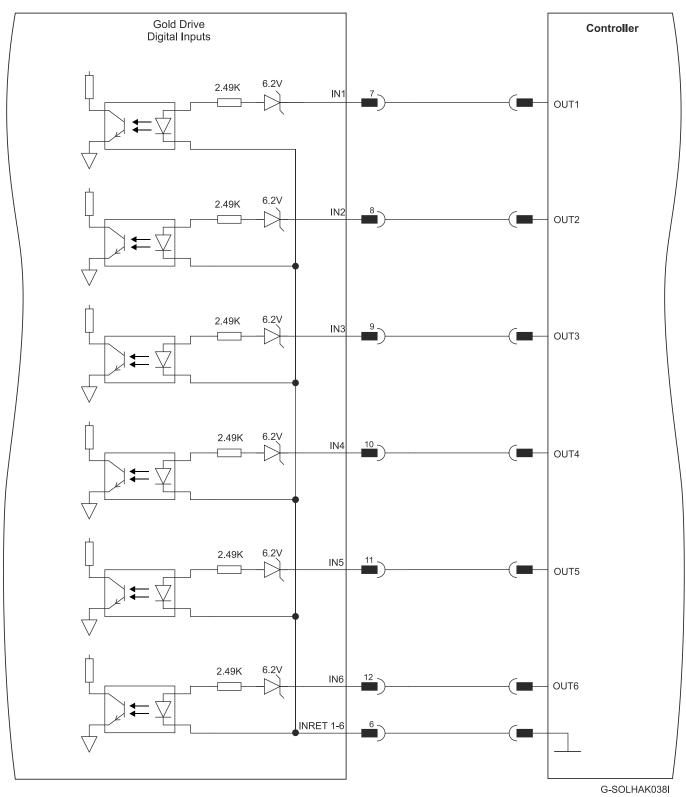
Figure 27: Digital Input Connection Diagram – Source PLC Option
