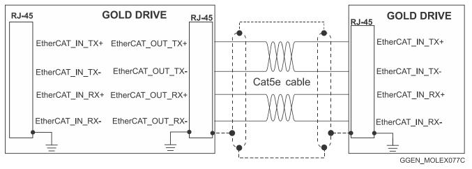
Figure 36: EtherCAT RJ-45 Connections
