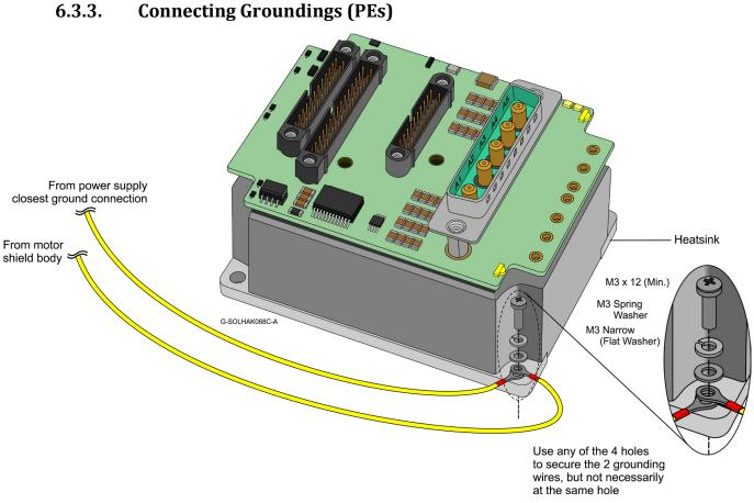
Figure 13: Connecting Groundings to the Heatsink
