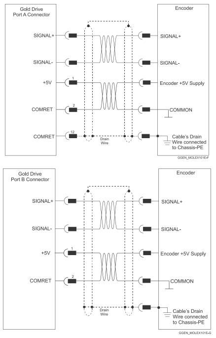
Figure 5: Feedback Port A and B Cable Assemblies
