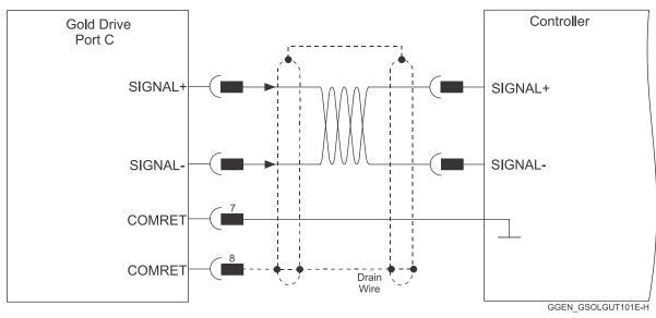
2. The connection of the Drain wire to the Port C is not mandatory.
