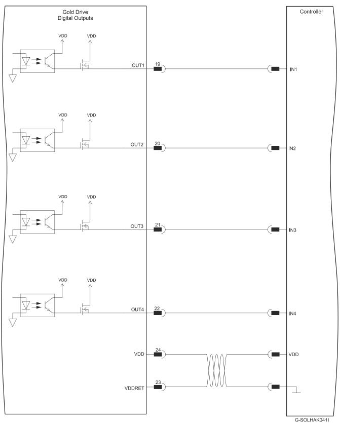
Figure 28: Digital Output Connection Diagram – Source PLC Option
