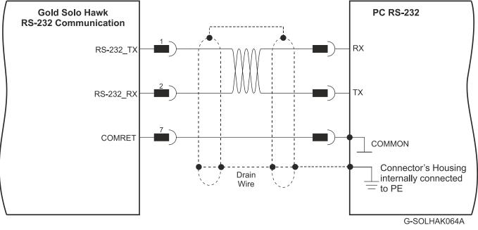
Figure 33: RS-232 Connection Diagram
