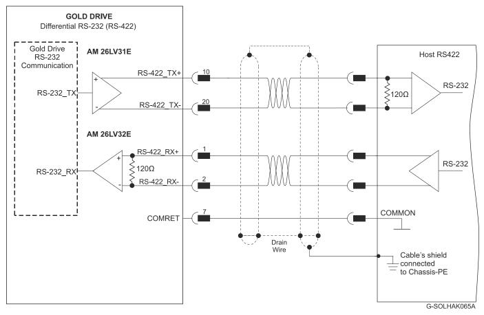
Figure 34: RS-422 Connection Diagram
