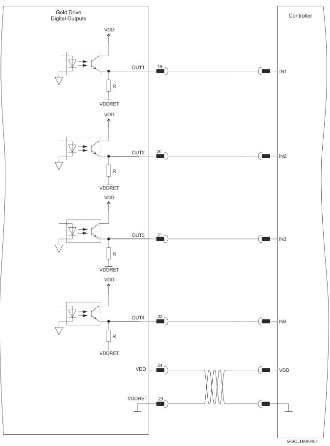
Figure 26: Digital Output Connection Diagram – TTL Option
