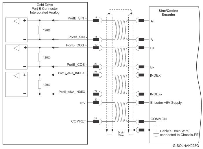
Figure 21: Port B - Interpolated Analog Encoder Connection Diagram
