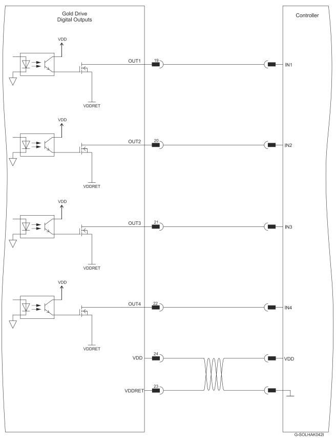
Figure 30: Digital Output as Sink Configuration Connection Diagram
