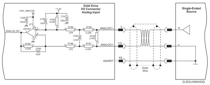
Figure 24: Differential Analog Input
