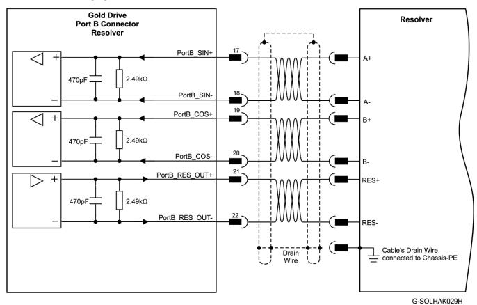
Figure 22: Port B – Resolver Connection Diagram
