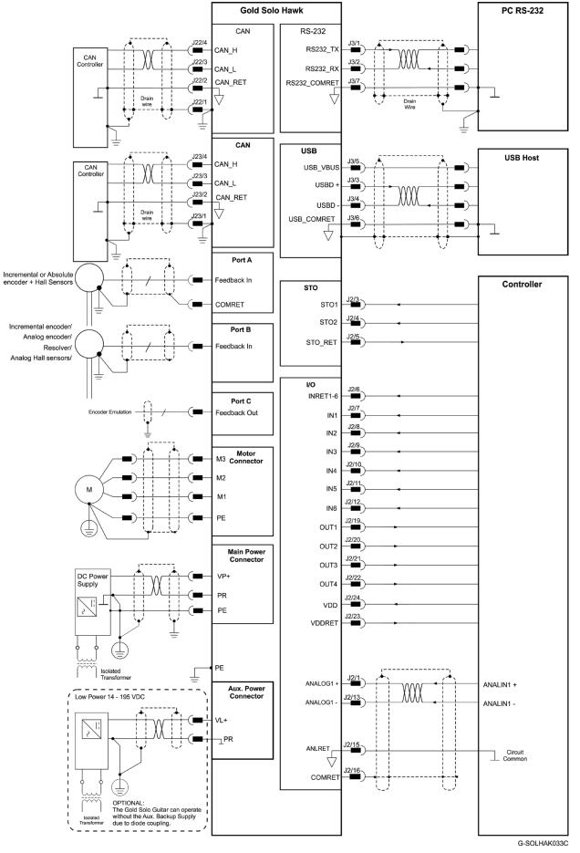
Figure 3: The Gold Solo Hawk Connection Diagram – CAN
