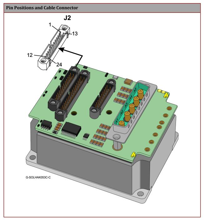
Table 7: Connector J2 – Digital I/Os, Analog Inputs, and STO Pin Assignments
